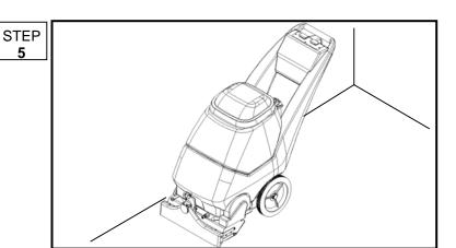
After cleaning, turn off all controls, return brush to storage position and carefully unplug machine.
